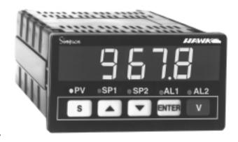
By using the password feature, the meter's programming functions and set points are protected from accidental reprogramming.
