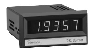
Simpson's 2842 Series meters offer high accuracy with up to 1nA resolution. Model 2842 requires a 120VAC power supply at 50-400Hz. The large 4-1/2-digit display is easily read from a distance of about 25 feet. Panel adapters are available for 1/8 DIN panel cutouts. In addition, a large "U" shaped mounting bracket is available for applications where the panel strength is unknown or weak.
