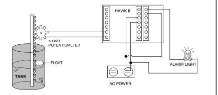
Hysteresis should be set at 5. This will prevent "chatter" in the relay, should the tank float bounce on the surface.
