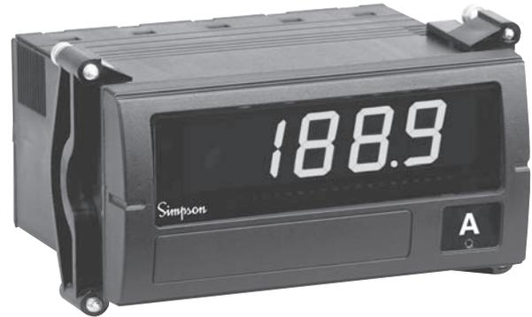
The Falcon Series digital indicators are premium quality 1/8 DIN meters for industrial applications. All Falcon units feature jumper-selectable decimal point (internal and on the connector for remote decimal point) and display scaling, providing wide application flexibility. In addition, most signal input ranges are easy to change with jumpers on the main board. The Falcon has a 0.56" bright red LED display for high visibility.
