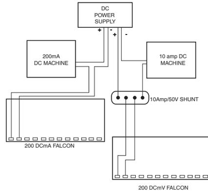
The shunt is installed in series between the source and the load, and the meter is connected to the shunt in parallel. The two lead wires included with the shunt are connected
