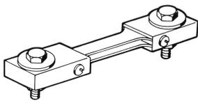
External shunts enable DC volt digital panel meters to indicate higher DC currents than can be provided with self contained internal shunt meters. The shunt is installed in series with the load and the source. The shunts provide a DCmV drop which is sent to the display unit. The Falcon can be scaled to display the current between the load and the source. Simpson manufactures portable and switchboard shunts.
