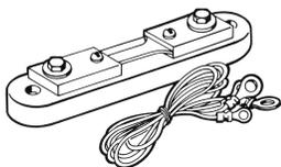
Each shunt includes 5' leads (0.065Ω resistance). Accuracy is within ±1% of rating.
