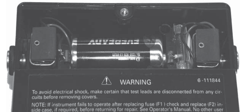
Figure 2. Rear View (Battery Cover Removed)
