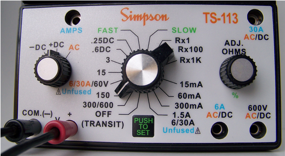
Figure 5. Measuring AC or DC Volts
