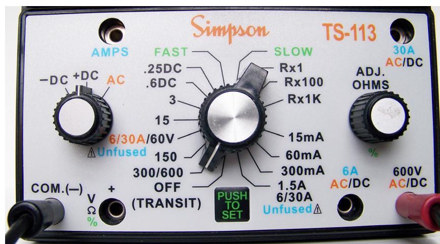
Figure 5a. Measuring High AC or DC Volts
