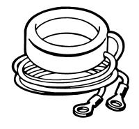
Donut Current Transformers enable the HAWK II to monitor AC current up to 1000 amps. The Donut (also known as a "Toroid") is placed around one of the legs of the device being monitored, and emits up to a 5 amp signal. The HAWK II can be scaled to accurately display the current being monitored. Each Donut comes with 2' long secondary leads.
